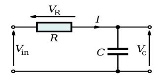
When capacitor fully charged, no current flows
