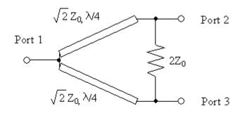
Phasing lines: delay signal to one antenna
