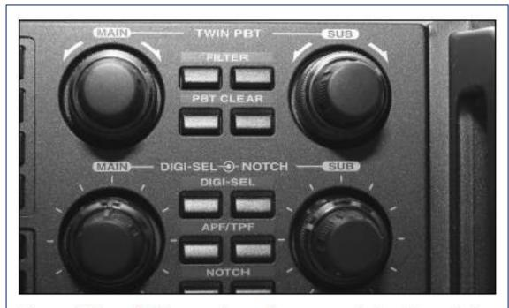
Figure 2.3 — HF transceivers have a variety of controls to help minimize interference on crowded bands. These may include notch filters, passband filters, audio peak filters and similar features.
