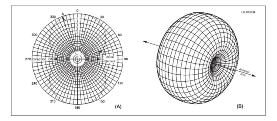
Part **A** shows the radiation pattern in the plane of a dipole located in **free space** Part **B** shows the three-dimensional radiation pattern in all directions around the dipole.
