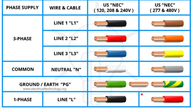
\* Use this in case of a Second Hot Wire i.e. in Single Phase, Two Lines 240V AC System.
