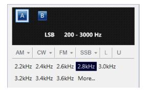
This windows shows both VFO-A and VFO-B are available, the current VFO being VFO-A. The current mode is LSB (lower sideband), the filter width is 2,800Hz (from 200 to 3000 Hz).
