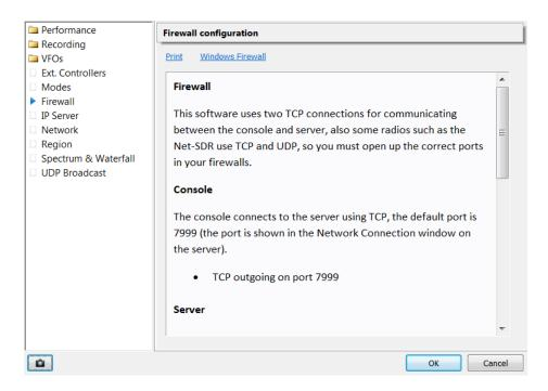
This software uses two TCP connections for communicating between the console and server, also some radios such as the Net-SDR use TCP and UDP, so you must open up the correct ports in your firewalls.
