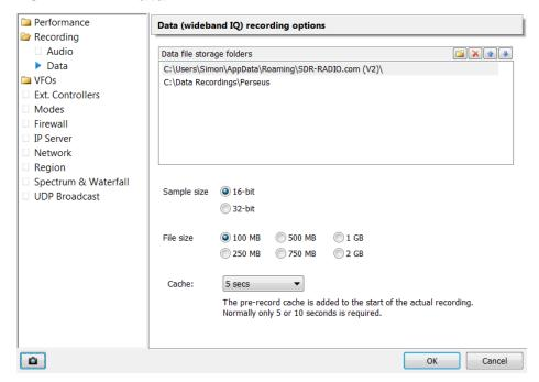
Data recordings contain the raw IQ data read from the SDR radio, this can be played back for later signal analysis.
