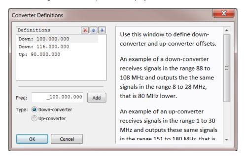
Use this window to define down-converter and up-converter offsets. Simply enter the frequency difference and select down-converter or up-converter.
