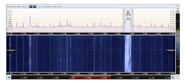
The main display window gives you a full overview of the signals in radio's span. To change the display span select an option from the Span button in the toolbar.
