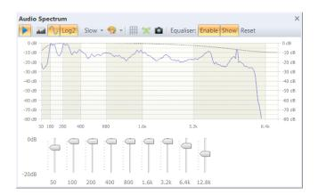
When you select the Show option the equaliser sliders are displayed, the slider range is 20dB. Graphical equalisers are implemented via a series of Biquad IIR filters, one filter per slider.
