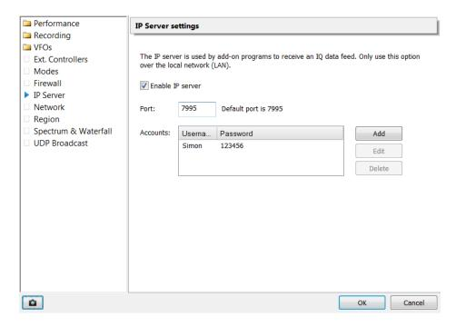
The IP Server provides support for add-on programs by sending an IQ data stream by sending data and control commands using TCP. The add-on programs connect to the console using the port and one of the accounts specified here.
