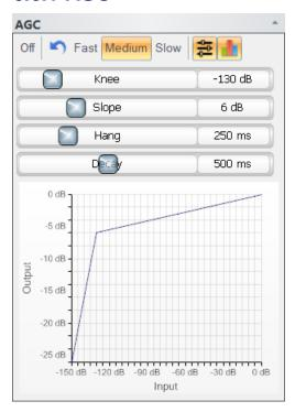
Automatic gain control (AGC) is an adaptive system found in many electronic devices. The average output signal level is fed back to adjust the gain to an appropriate level for a range of input signal levels. For example, without AGC the sound emitted from an AM radio receiver would vary to an extreme extent from a weak to a strong signal; the AGC effectively reduces the volume if the signal is strong and raises it when it is weaker. (From Wikipedia, the free encyclopedia.)
